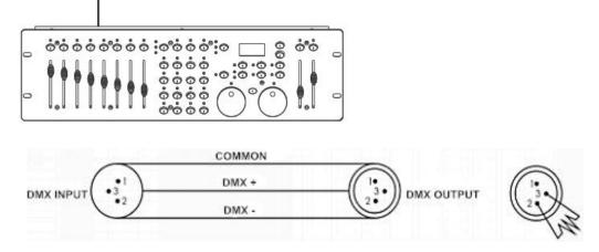
Termination reduces signal errors and avoids signal transmission problems and interference. It is always advisable to connect a DMX terminal. (Resistance 1290hm 1/4 W) between pin 2(DMX-) and pin3 (DMX+) of the last fixture.
